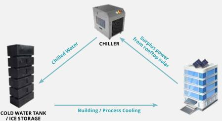
Chillers can be controlled to cool storage tanks down to their lowest temperature during low energy cost periods (or to use surplus solar generation on site) and turned off/down during high energy cost periods, so that the load is met from the stored cold in water or ice.
