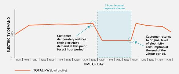
Figure 1 provides an illustration of 24 hours of electricity demand within a commercial building. At 1:30pm it participated in demand response, reducing its electricity demand for 2 hours by shutting off various plant, such as air conditioning. The demand response period is shown by the shading.
